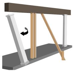
When replacing an existing column, place a temporary support beside the column you are planning to replace. Use a 4x4 or 2x6 and a bottle jack if necessary to make sure the load is properly supported. Once the load is supported remove the old column.
