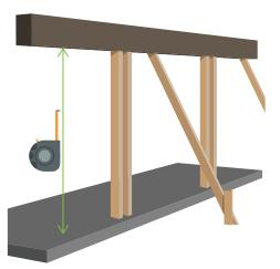
With proper bracing in place in "new" construction, measure the distance from the floor to the header support.
