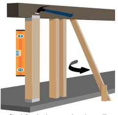
Check for plumb, ensure the column will support the load, then secure the top and bottom of the column. If using a metal connector, refer to manufacturer's instructions. Remove the temporary bracing.
