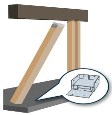
Attach the plinth or metal connector to the bottom of the Culpeper Columns and slide the column into place. If a high wind tie-down cable or rod is required, consult code and manufacturer's recommendations.
